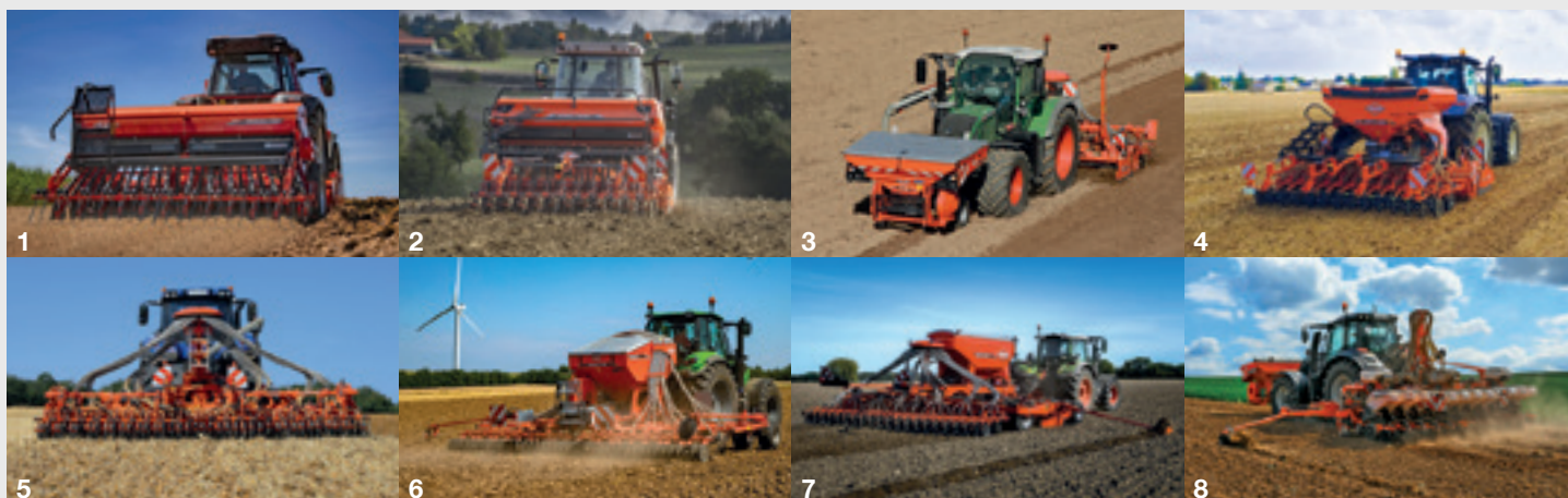
1. Mounted mechanical - 2. Integrated mechanical - 3. With front hopper - 4. Integrated pneumatic - 5. Foldable pneumatic 6. Mounted for min-till - 7. Trailed for min-till - 8. Precision seed drills
