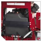
Generous 7.75-gallon fuel tank is centrally located for consistent balance, and the fuel filler neck is conveniently located on the side for easy filling.
