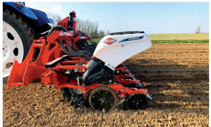
Row shut-off per GPS is operated by shutting down the motor on each row, in a very reactive manner and without seed loss. This ensures farmers save significantly on seeds. By eliminating the wheel slip caused by the soil conditions, the electric drive ensures a perfect seed application rate.
