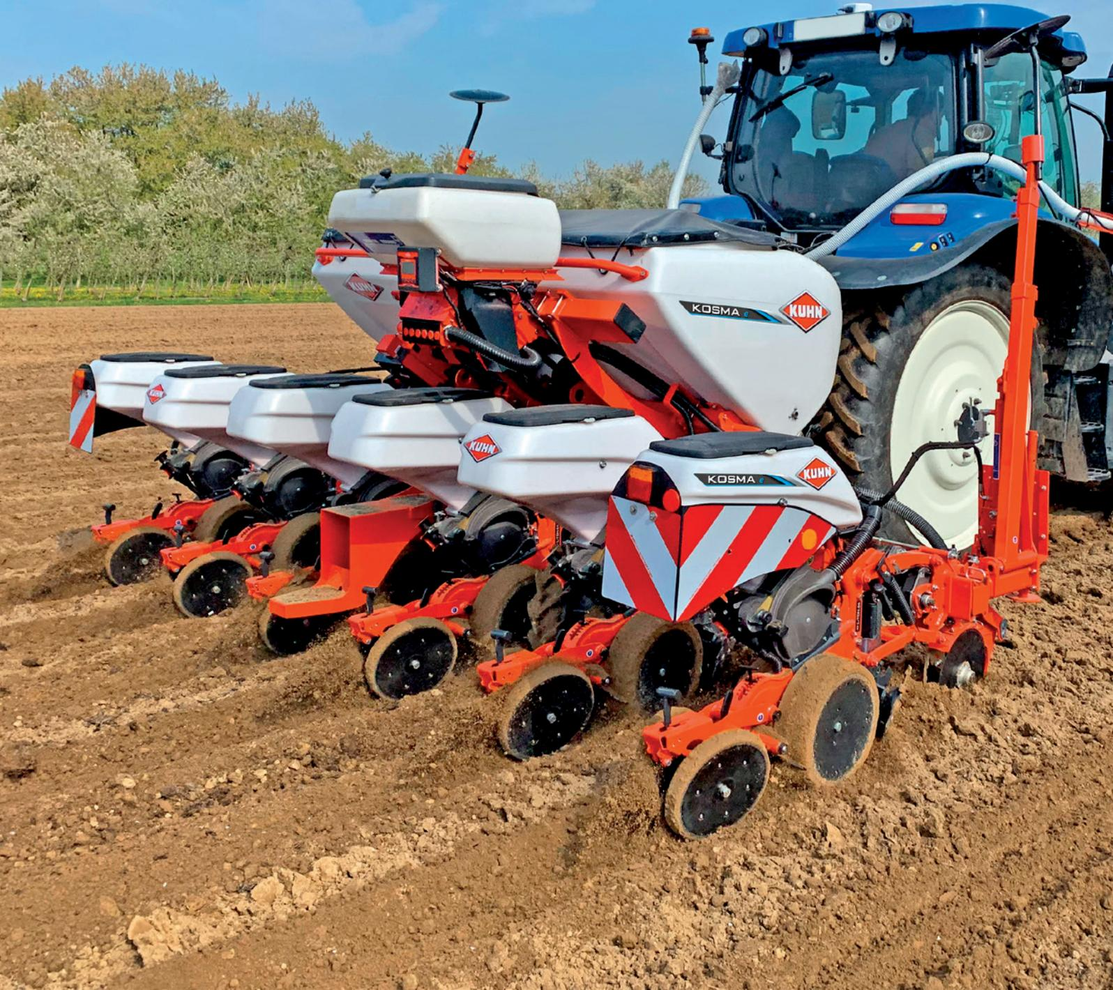
Designed for a transport width of only 3 metres, the KOSMA version of this chassis lets farmers seed 6 rows with 75 cm spacing. The MAXIMA 3 version is fitted with a larger frame to accommodate up to 1,350 litres of fertiliser. It drills up to 6 rows at 80 cm spacing.
