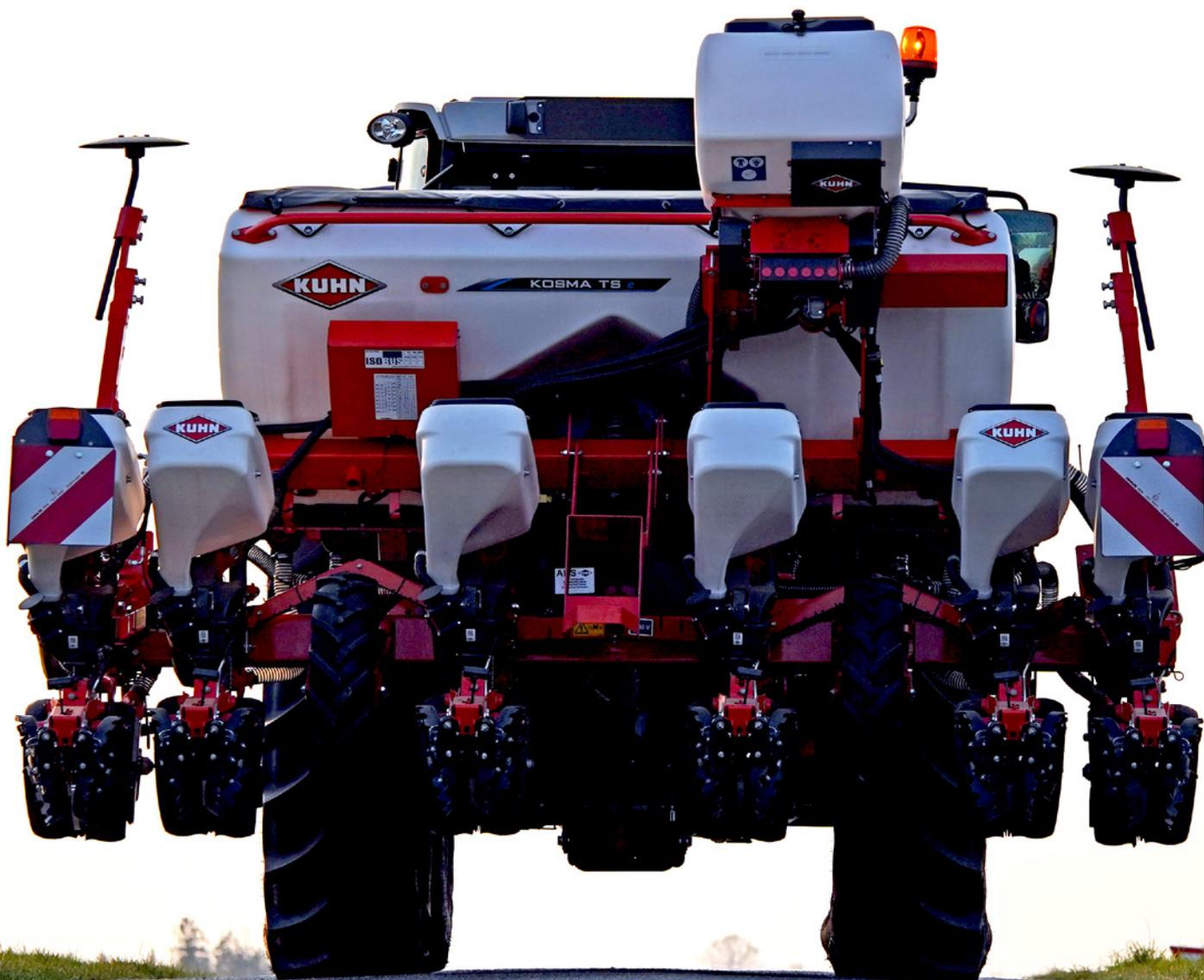
Work at widths of up to 4.5 metres with reduced transport widths between 3.3 and 3.5 metres, depending on row spacing. That's what the telescopic single bar chassis offers via a simple and robust slide link. This best-seller owes its success to its robust build and simplicity.
