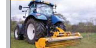
Min 50hp • Max cut width 2.8m
