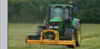
Min 50hp • Max cut width 2.65m
