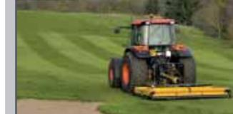
Min 70hp • Max cut width 2.6m
