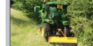
Min 35hp • Max cut width 1.5m
