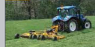
Min 80hp • Max cut width 4.6m
