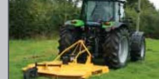
Min 20hp • Max cut width 2.1m
