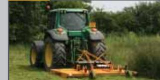
Min 50hp • Max cut width 2.75m
