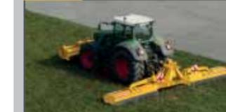
Min 220hp, Max cut width 8.0m
