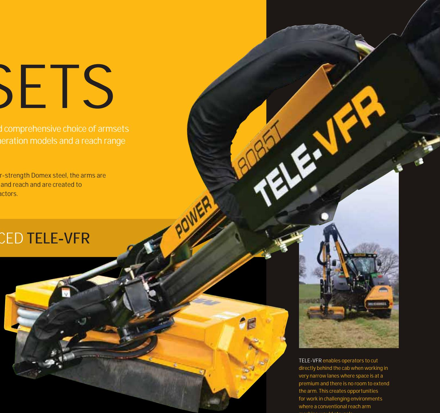
TELE-VFR enables operators to cut directly behind the cab when working in very narrow lanes where space is at a premium and there is no room to extend the arm. This creates opportunities for work in challenging environments where a conventional reach arm machine would struggle.
