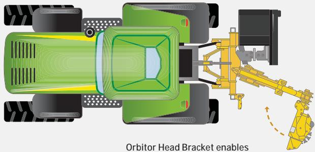
Orbitor Head Bracket enables an extra angle of movement
