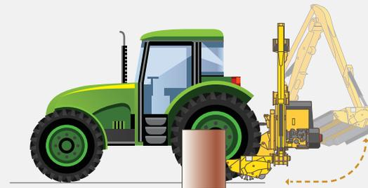
Hydraulic safety breakaway enables the Power Arm to break backwards and upwards on contact with an obstacle
