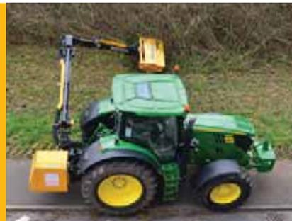
Arm can be positioned alongside the cab
