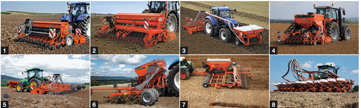
1. mounted mechanical - 2. integrated mechanical - 3. with front hopper - 4. integrated pneumatic - 5. mounted seeding combination 6. mounted min-till - 7. trailed min-till - 8. precision seed drills
