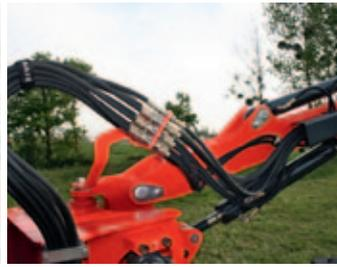
**❸ Hose routing** designed for optimum protection. All arm hoses are integrated into a protective casing. A swivelling and rotating hose support plate reduces friction phenomena at the pivot.
