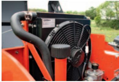
**❷ A 12 kW air-cooled radiator** as standard for constant power. All hydraulic components are protected against temperature peaks.
