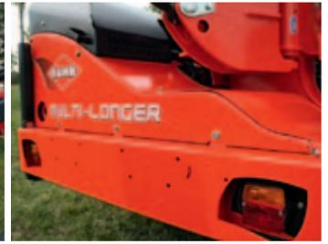
**❹ Full enclosure.** Over and above aesthetic aspects, the frame on the MULTI-LONGER GII range is fully encased to guarantee full machine component protection. The frame has four storage stands and incorporates a bumper with integrated lights.
