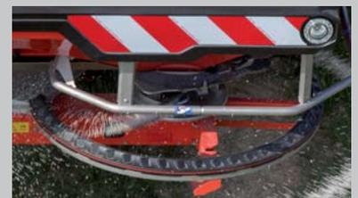
**AXMAT duo:** Radar-supported, automatic spreading pattern control
