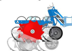
Individual lifting by manual or automatic GPS-controlled hydraulic control
