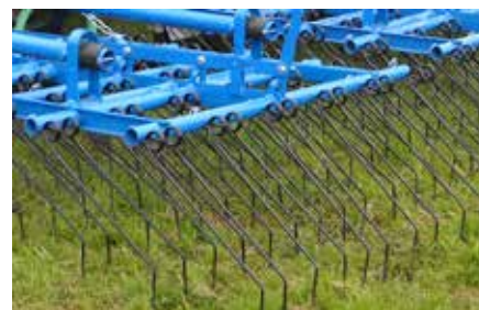
Ø 8mm compact (L=530mm) Efficient moss take off
