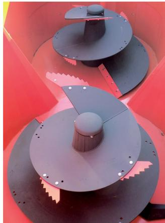
For SPW Intense 19, 22, 25 and 27 m<sup>3</sup>: hydraulic engine drive system allowing for improved chopping of the fibre and optimum cleaning at the end of feeding, coupled with a rigid connection between the 2 augers. The speed can be adjusted from 0 to 55 rpm. No maintenance required.
