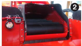
To boost the loading rate of this new range of self-propelled mixer wagons, the width of the loading conveyor has been increased from 650 to 800 mm (3). The fodder flow transits quicker between the milling head and the mixing hopper.
