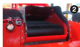
To boost the loading rate of this new range of self-propelled mixer wagons, the width of the loading conveyor has been increased from 650 to 800 mm (3). The fodder flow transits quicker between the milling head and the mixing hopper.
