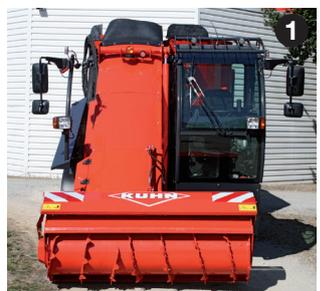
The loading conveyor has been totally redesigned! First of all, in terms of its drive. The belt is now driven by a hydraulic motor at the top of the conveyor (2). As a result, the belt is drawn by the motor which helps to centre it. Centring is further assisted by a thin strip on the belt that slots into a groove in the driving rollers. The belt is therefore always correctly positioned in the middle of the conveyor, thus avoiding the risk of side wear.
