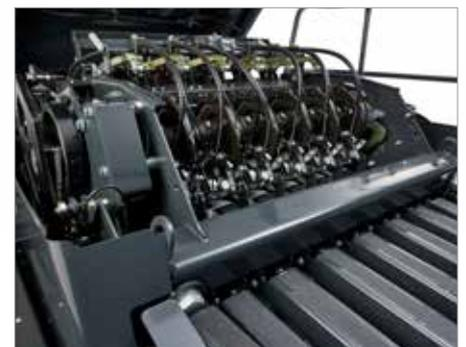
4. Double knotting system with standard electronic monitoring
