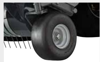
Semi-pneumatic pivoting pick-up guide wheels
