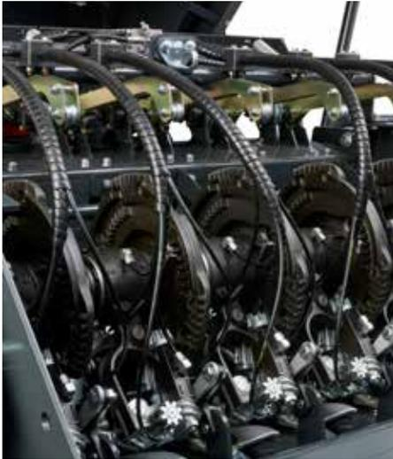
1. Double knotting system with standard electronic monitoring
