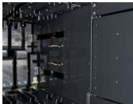
3. Replaceable, high wear-resistant bale channel parts.
