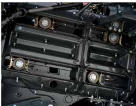
2. Heavy-duty, greased plunger rolls
